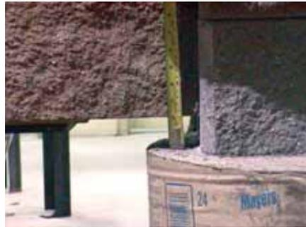
A two part objective. The first to prove the load carrying capabilities of a panel assembly that is simply supported by the panels resting on simulated piles at the posts. Second, to establish the ability of the post and panel structure to handle loads exerted on the panels from the underside.
