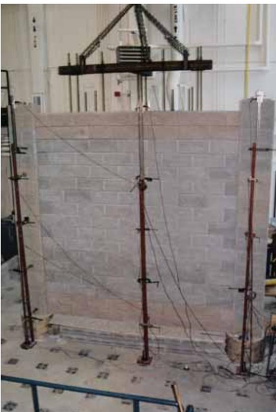
*Flexural Test Setup Structure C*
