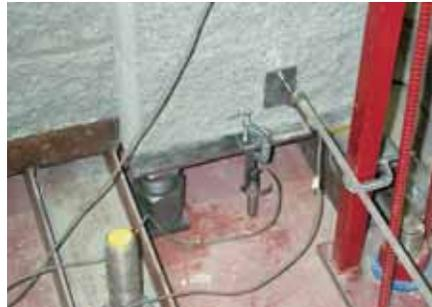
*Displacement Transducers Measuring Rotation*
