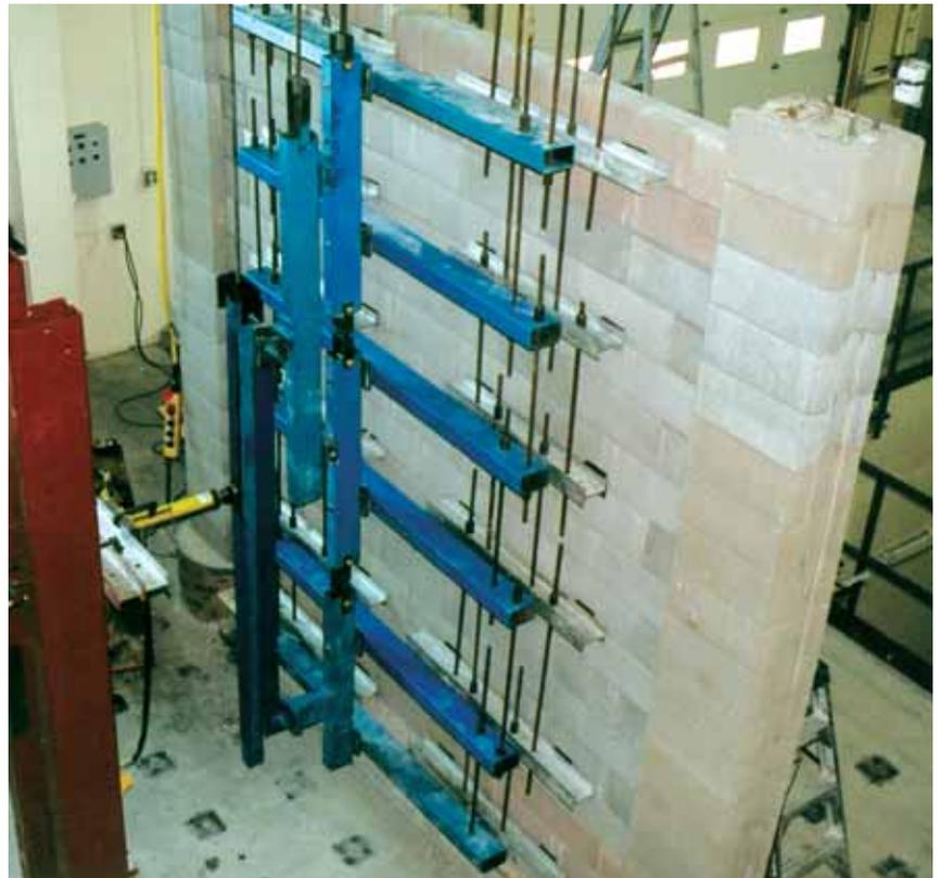
*Flexural Test Setup Structure C
