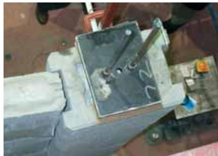
*Post-Tensioned Masonry Posts*
